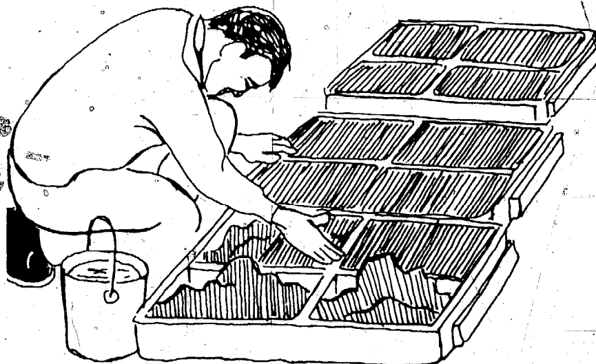
Figure 40. Kneading and leveling the blocks.
